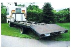
The ramps to drive cars onto the flatbed were pretty shabby. Each of the two ramps was constructed of two 8" X 2" Steel Channels welded together at the centers. Years of corrosion had caused the ramps to warp at the centers, so, the ramps were separated, ground to bright metal, painted with "Rust X" (a rust encapsulation material), and welded back together.
