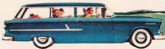
THE "TWO-TEN" HANDYMAN —At work or at play, this 2-door Station Wagon is a pleasure to look at—a joy to drive. Front-seat backs swing way up for easy access to rear seat and cargo area. Interiors—even roof linings—are of colorful, tough and easily washable vinyl.
